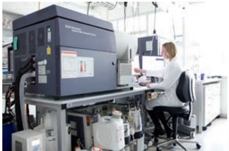
Figure 2. BD FACSAria, a high-speed benchtop cell sorter used to sort fluorescent cells into tubes and multiwell plates.
