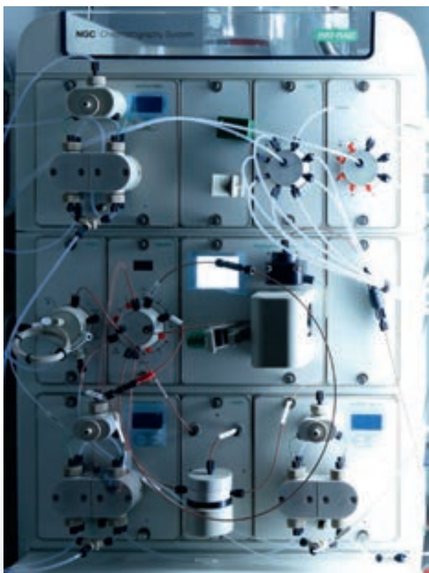
Figure 1. The Biorad NGC Quest Plus chromatography system is the new workhorse FPLC within the PPCF. It is located inside a cooling cabinet and offers a high degree of versatility. Semi-independent workflows are possible due to an additional sample pump, multiple inlet and column switching valves, an air detection system, as well as a fractionator that allows sample collection from microtiter plates to 250 ml bottles.
